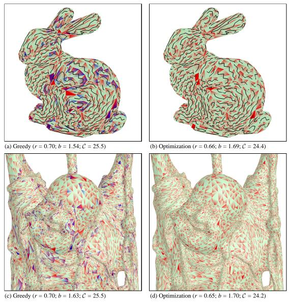
Figure 9: Results of greedy strip-growing (left column) and local optimization (right column) with a 16-entry FIFO vertex cache, for bunny 2000 and buddha. (Blue corners on the left indicate cache misses eliminated on the right.) Captions refer to the average number r of cache misses per triangle, the strip bloat factor b, and the overall bandwidth cost C in bytes per triangle.
