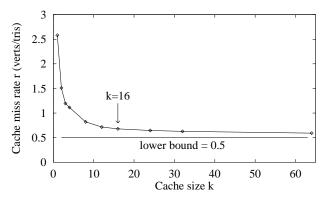
Figure 8: FIFO cache effectiveness as a function of cache size with the greedy strip-growing algorithm on the 4000-face bunny.
